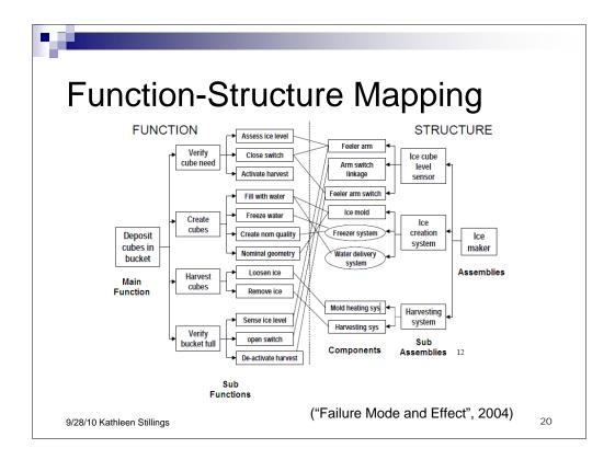
An alternate decomposition method which can be used to assign dependencies.
